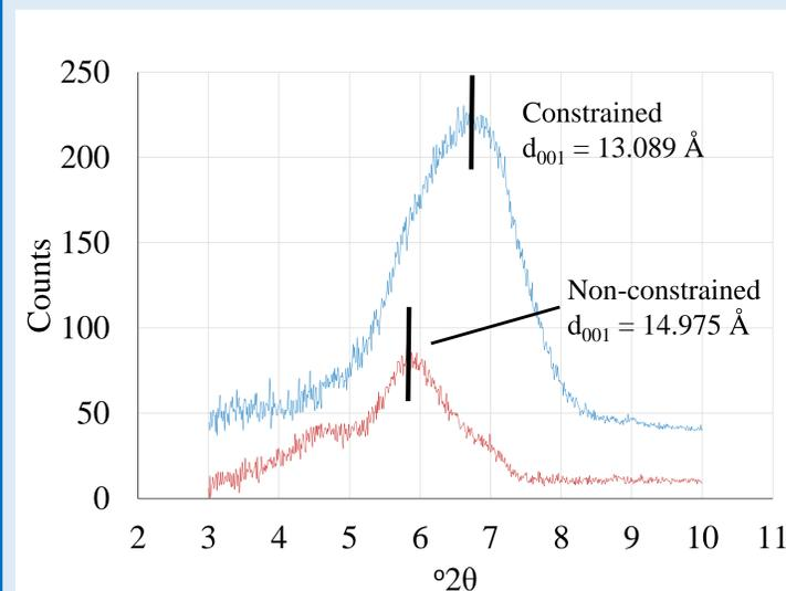
**Figure 4.** X-ray diffraction of montmorillonite in constrained and non-constrained environments.
