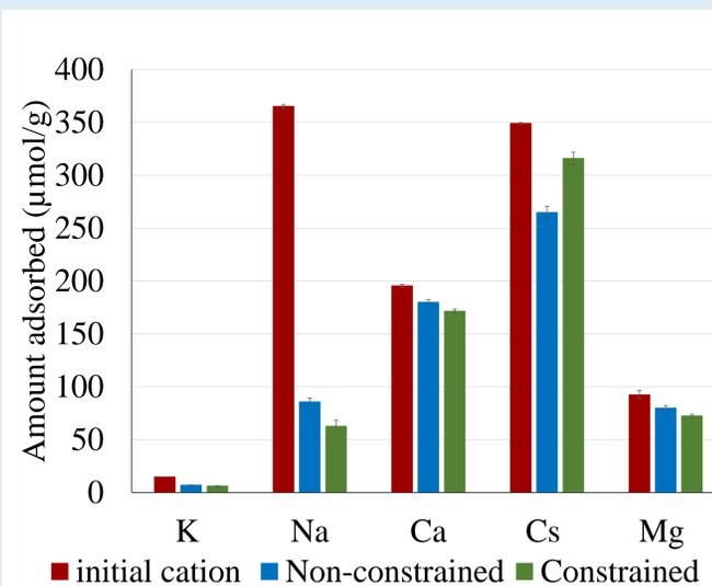
**Figure 3.** Cation adsorption on montmorillonite in constrained and non-constrained environments.
