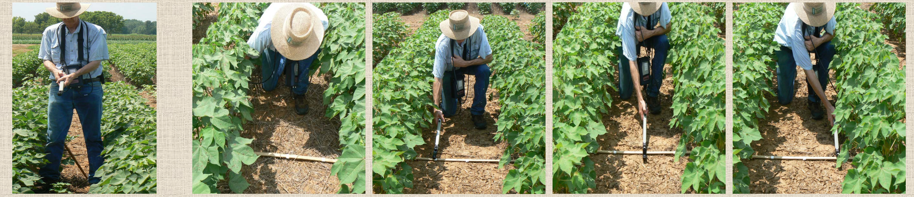
Above-canopy Measurement Four Below-canopy Measurements Parallel to the Row and at 0, 1/4, 1/2, and 3/4 the Distance in Middle
