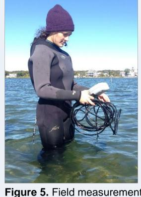
of DO, temperature, salinity, and pH were taken using YSI
