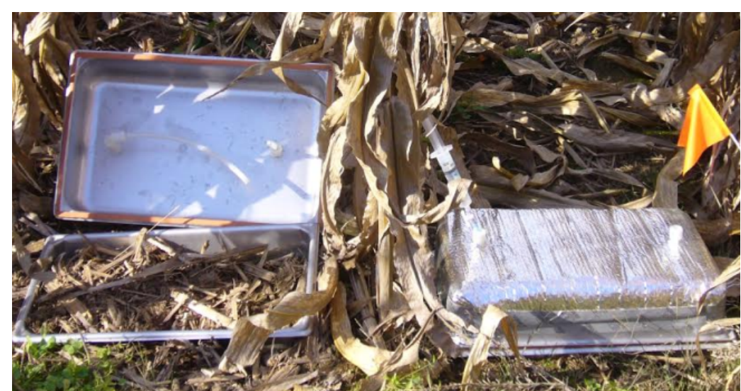
Fig. 1 Two chambers in each treatment-plot
