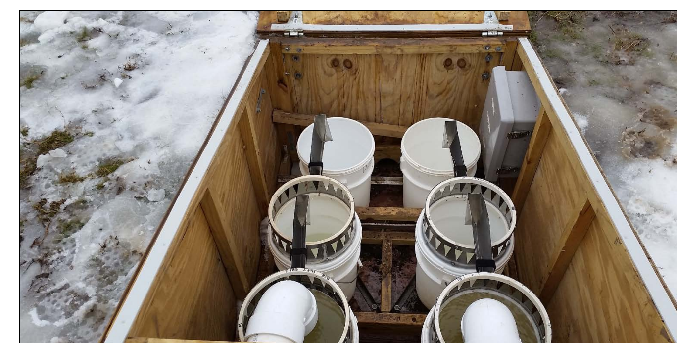
A passive-divider runoff collection system uses V-notch weirs to collect up to 15 cm events for water analysis and load cells to record flow rate.
