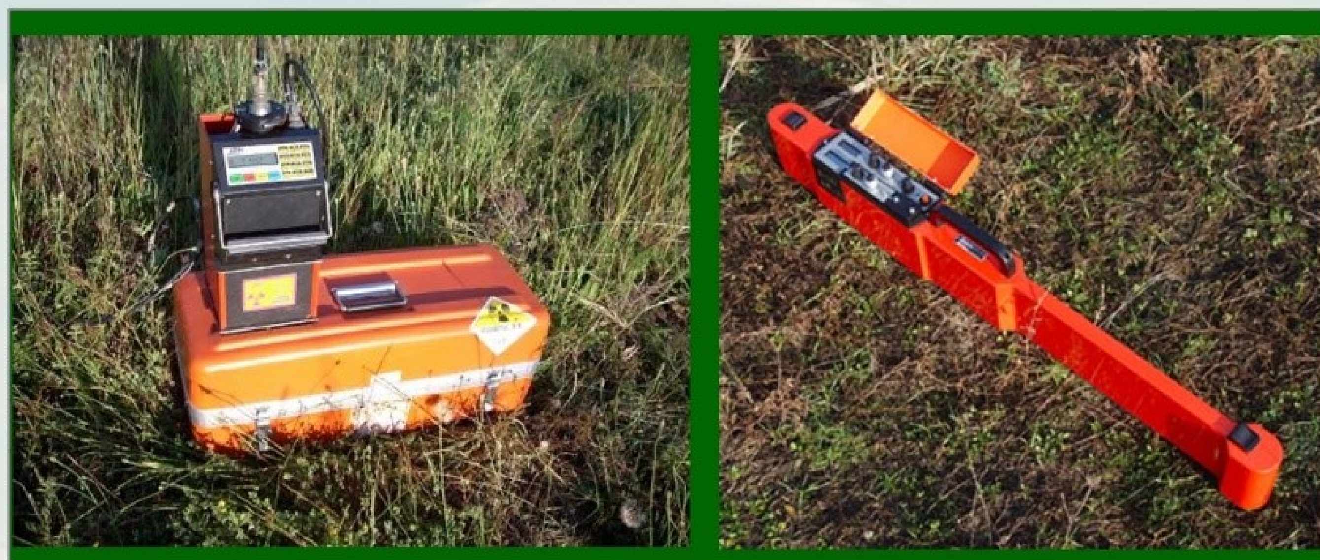
Fig. 1. Model 503 DR Hydroprobe for soil water content data collection (left). Geonics EM38-MK2 sensor for apparent electrical conductivity measurement (right).
