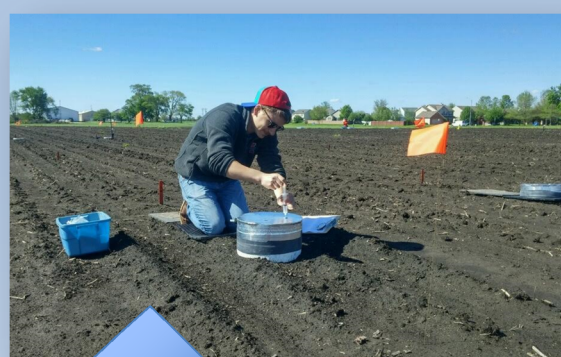
Field N 2 O fluxes measured using static flux chambers
