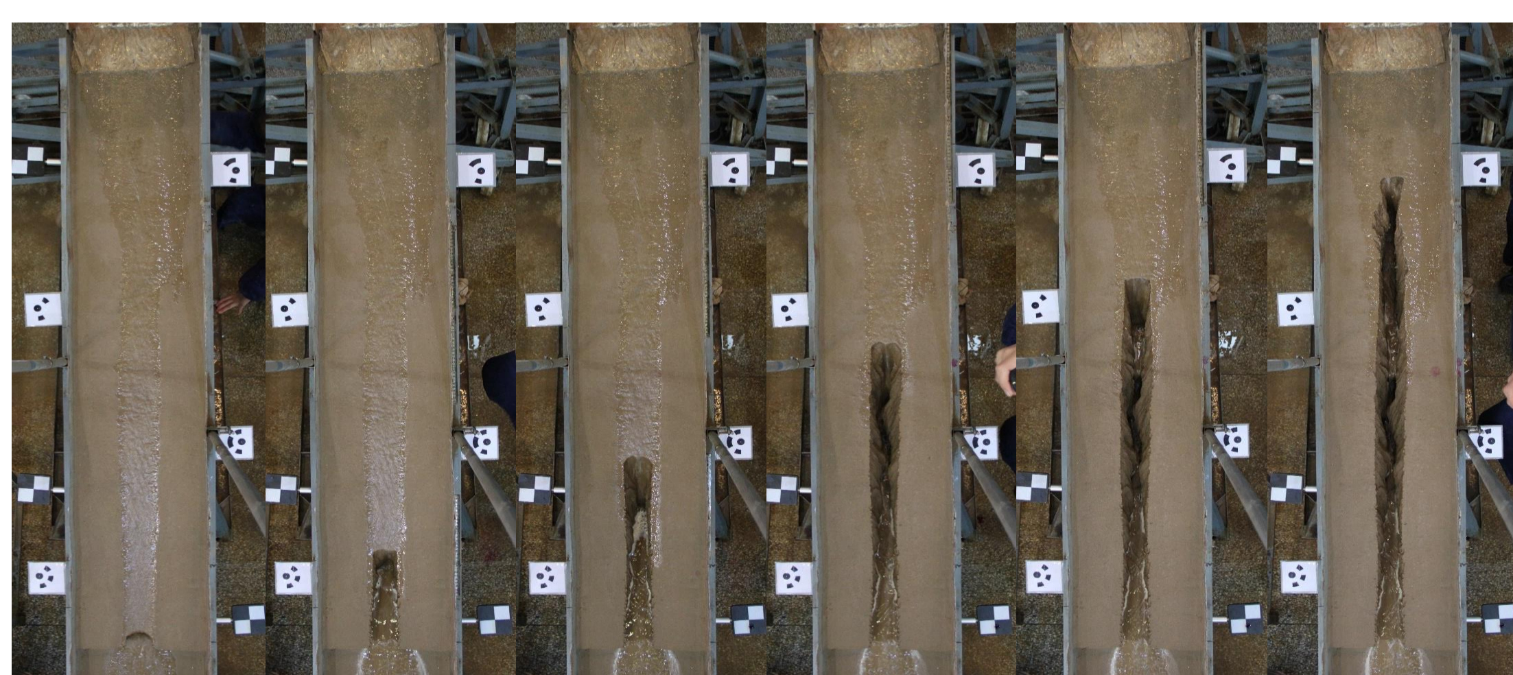
Fig. 2 Development processes of a well developed rill channel.
