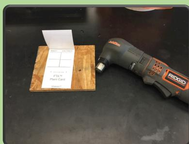
Collection: Samples are crushed onto an FTA-card using an auto-hammer and a wood support.
