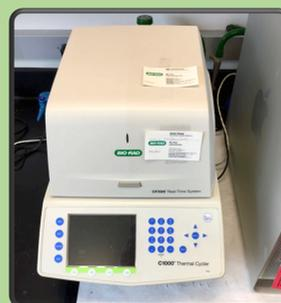
PCR: Bio-Rad CFX-96 machine was used for RT-PCR with Eva-green as the detection dye.
