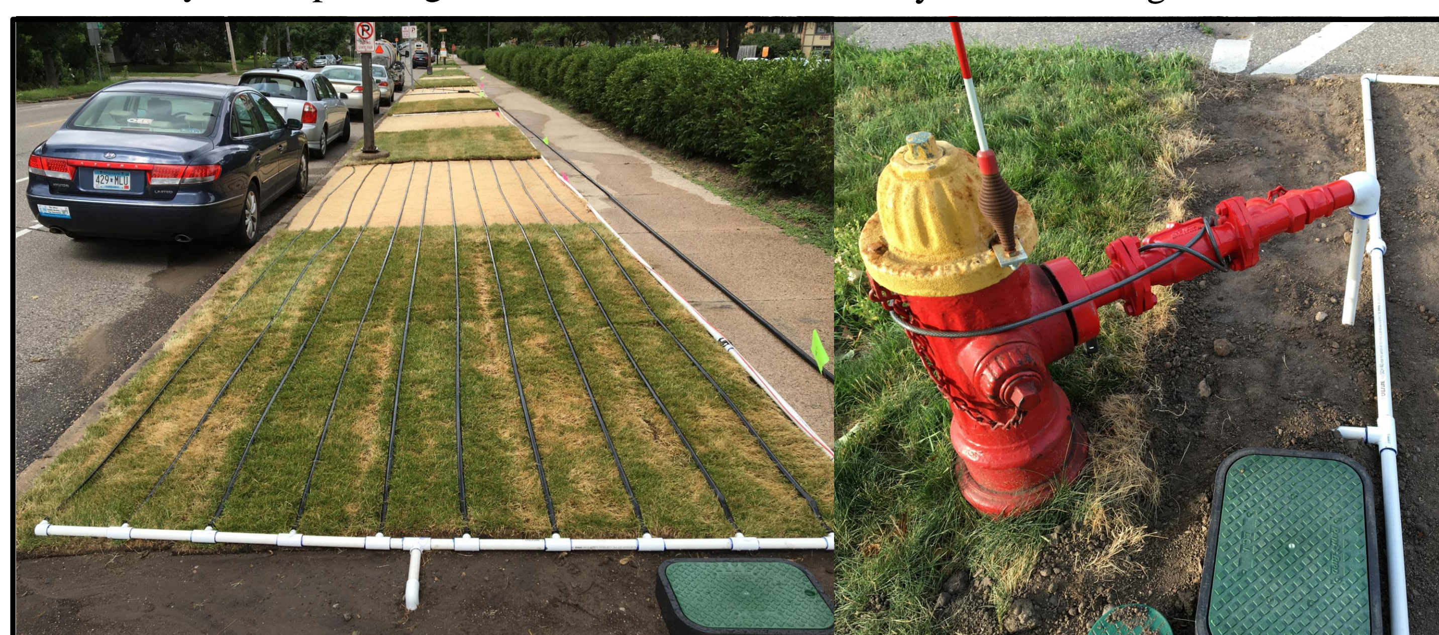
Figure 1. Location 2 trial area and example of fire hydrant connection
