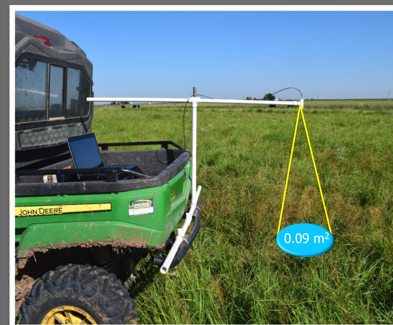
Figure 1. Sensor mounting design for spectrometer creates 0.09-m 2 sensing footprint.
