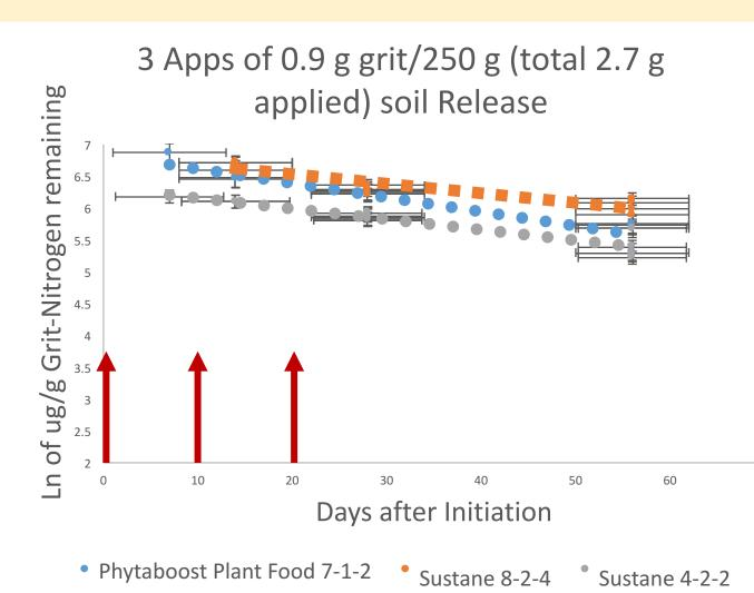
Figure 6. Natural log regression of nitrogen when 0.9 g was applied over a 20 d period, simulating 3 in-field grit applications. Arrows depict when grit was applied.
