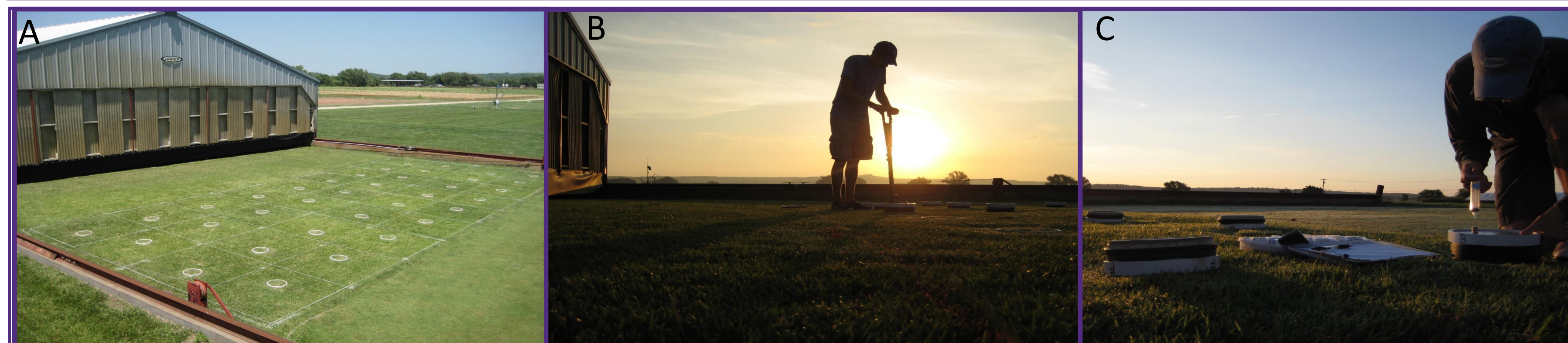
Figure 1. (A) Study area with the automated rainout shelter currently not covering the plots; (B) Recording volumetric soil water content of a plot with a time-domain reflectometry handheld meter while sampling N_2O ; (C) Sampling N_2O on DOY 174.
