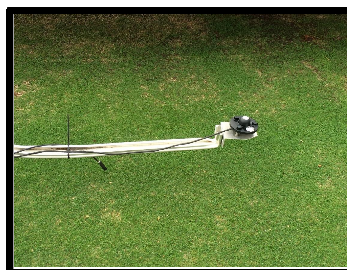
Fig. 2. Quantum light sensor mounted under each shade level to record daily PAR light integrals.
