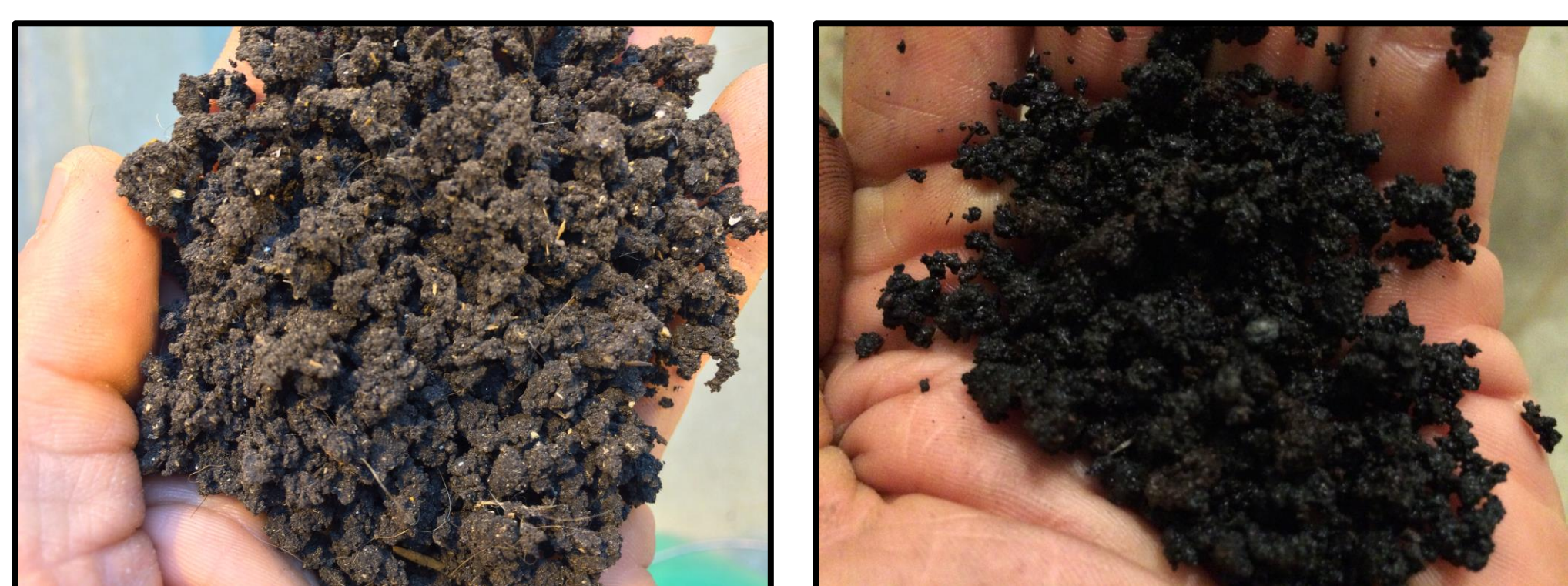
Figure 2. Dried biosolids (left) and biochar made from biosolids (right).
