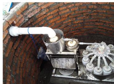
Figure 3. Runoff-Sediment Monitoring Device
