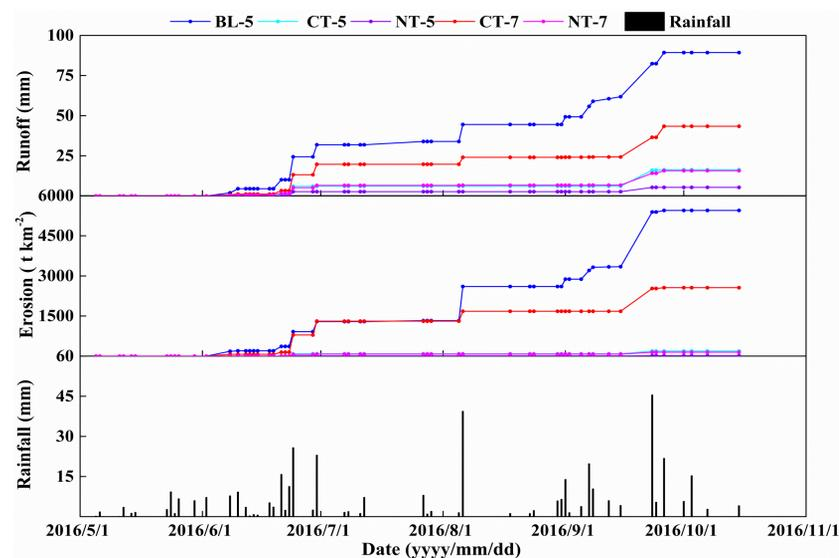
Figure 4. Cumulative surface runoff (mm) and soil loss (t km<sup>-2</sup>) of each combination of the tillage treatment and slope gradient over the period May 1st-October 30th, 2016. (BL-5: Bare land on 5° slope gradients; CT-5: Conventional tillage on 5° slope gradients; NT-5: No-tillage on 5° slope gradients; CT-7: Conventional tillage on 7° slope gradients; NT-7: No-tillage on 7° slope gradients)
