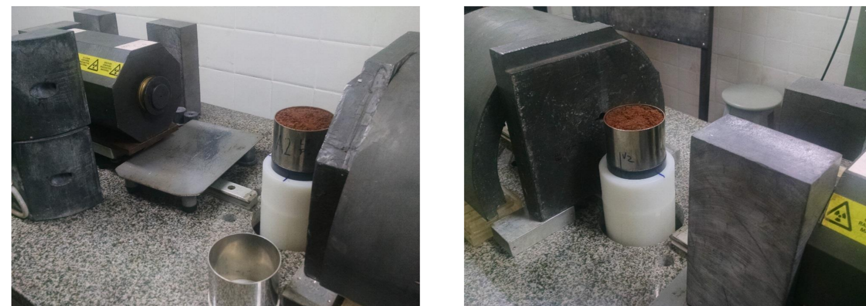
Figure 1 – Experimental setup showing a soil sample and \gamma -ray collimator
