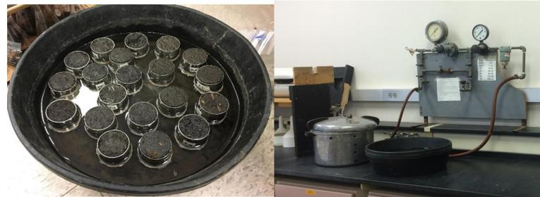
Fig.3. Core samples and ceramic pressure plate for water retention
