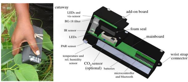
Figure 1. MultispeQ device in use
