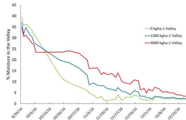
Fig. 3. Volumetric soil water content in the PAM band (valley) for 0, 1500, and 3000 kg PAM ha<sup>-1</sup>.
