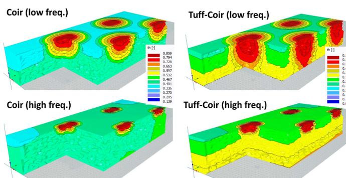
Figure 4. Water content distribution after low and high irrigation frequencies for coconut coir (left), and for the tuff-coconut coir mixture (right).
