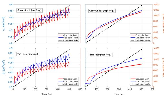
Figure 5. Left axis: volumetric water content at two observation points in the center of the container at 5 and 15 cm depths from the soilless substrate surface; Right axis: cumulative root water uptake for both substrates and two irrigation frequencies.
