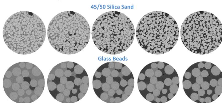
Figure 1: Sample cross sections of raw X-ray CT grayscale data for investigated silica sand and glass beads at various liquid saturation levels.
