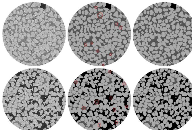
Figure 3: Comparison of KM (middle column) and KM-MRF (right column) segmentation. Raw data are in the left column.
