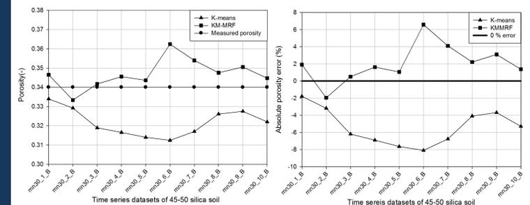
Figure 4: Comparison of actually measured porosity with porosities derived from segmented CT time series data for 45/50 silica sand (left). Relative porosity errors for the same time series dataset (right).
