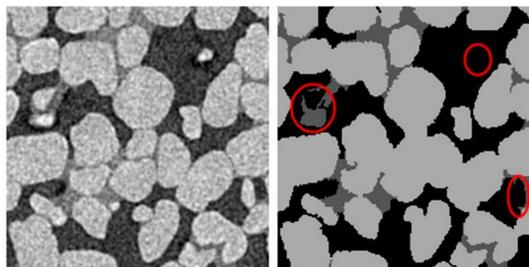
Figure 2: Example for misclassification errors of K-means clustering. Raw grayscale data (left) compared with K-means segmentation results (right).
