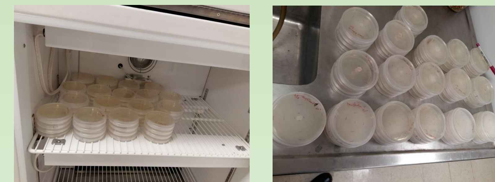
Figure 3. Incubation of cultures in growth chambers at 6 temperatures (10 to 40C)
