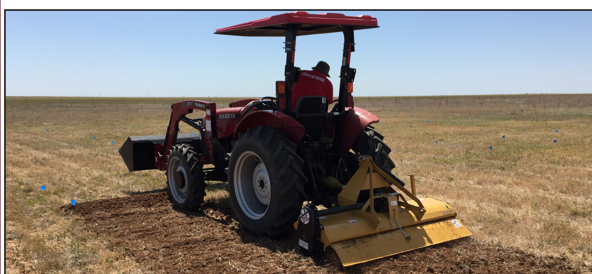
Figure 1. Tillage was completed using a PTO driven rotary tiller. Planting in 2016 was into native grass rangeland.
