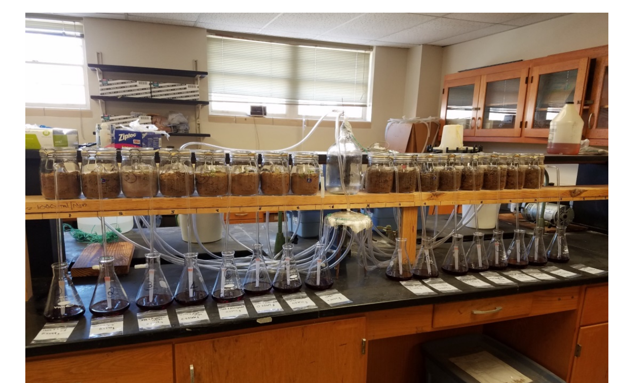
Figure 1. Laboratory bench procedure for determining ammonia loss from fertilized turfgrass, following the procedure of O'Halloran, 1993.
