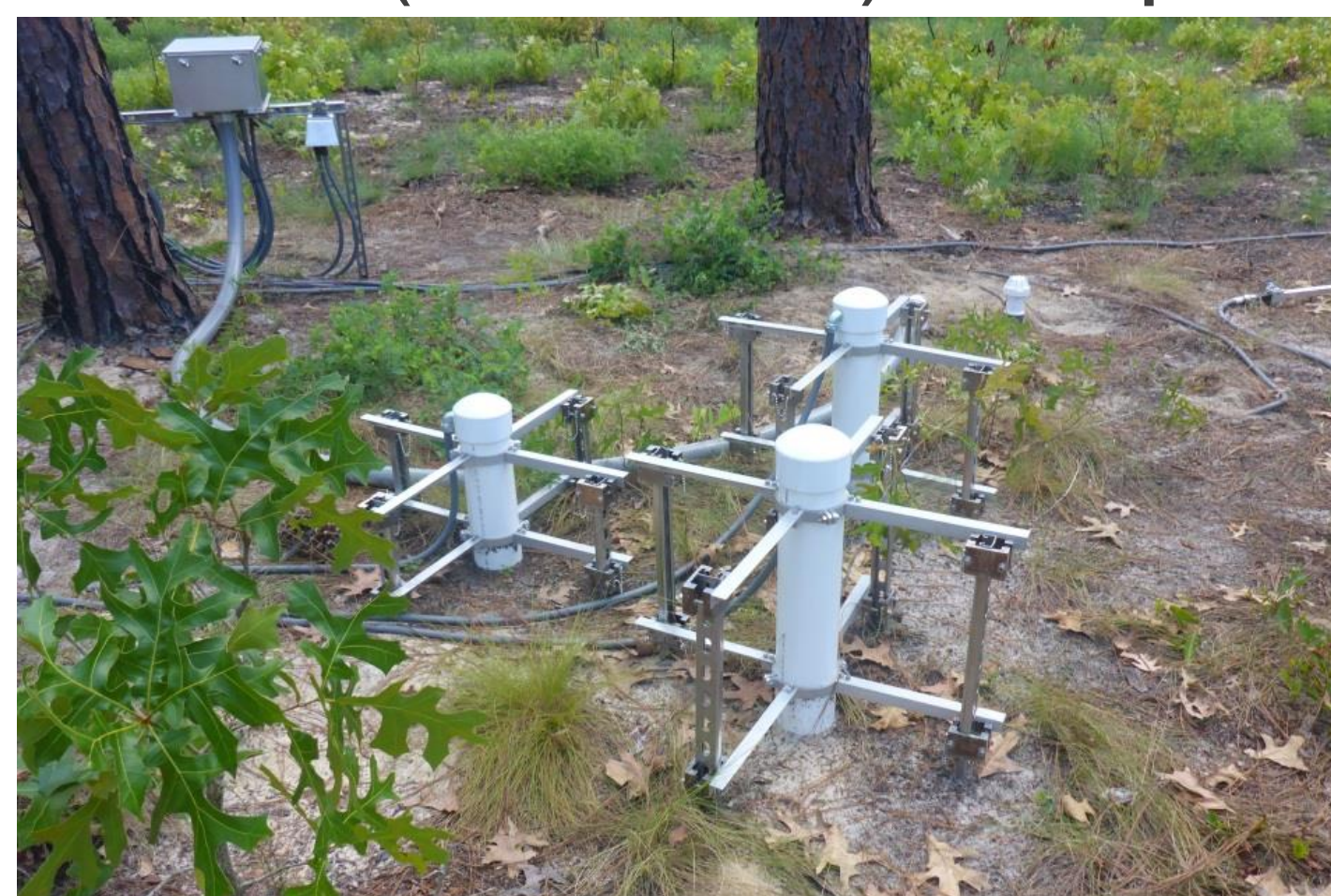
Fig. 1. Soil CO 2 assemblies measuring CO 2 concentrations at 3 different depths at Ordway-Swisher Biological Station, FL.
