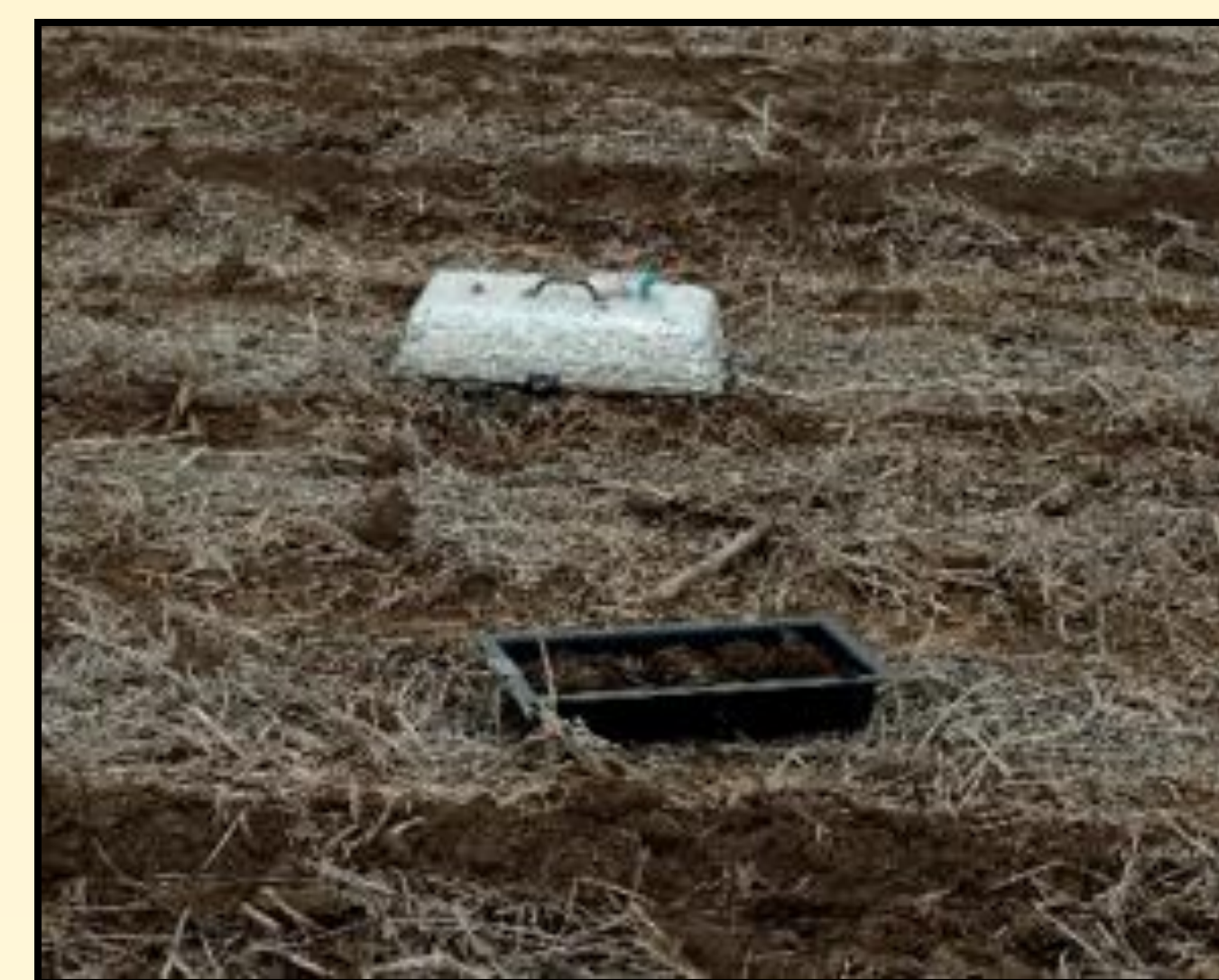
Fig. 2. Gas chamber used to collect gas samples
