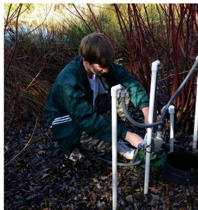
Taking a water sample from the lysimeter
