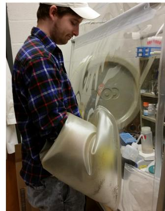
Preparing ferrozine-standard recipe in the glovebox in order to complex  $Fe^{2+}$  in the field
