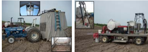
Figure 1. A welded frame surrounded with a wind screen, a top-mounted water nozzle, an electric bracket/clutch, and two return pans for excess source water return via a small transfer pump.
