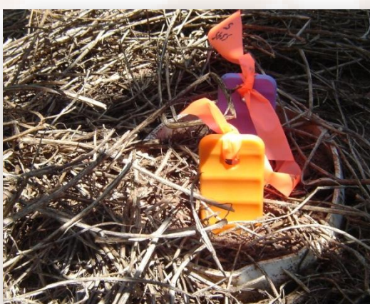
Top: PRS probes were placed in soil under rolled cover crop mulches
