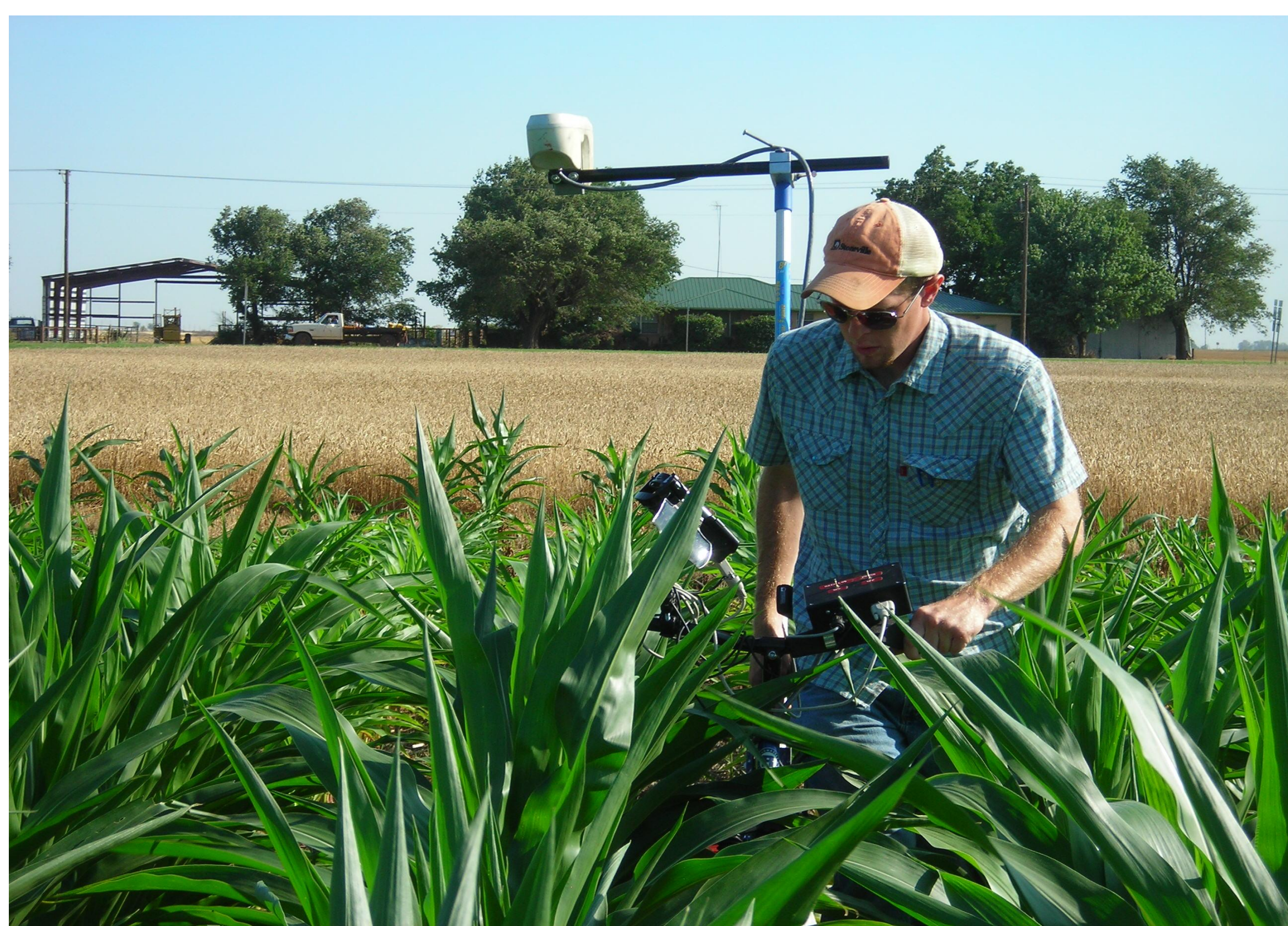
Figure 1. Reflectance measurement using the bike sensor
