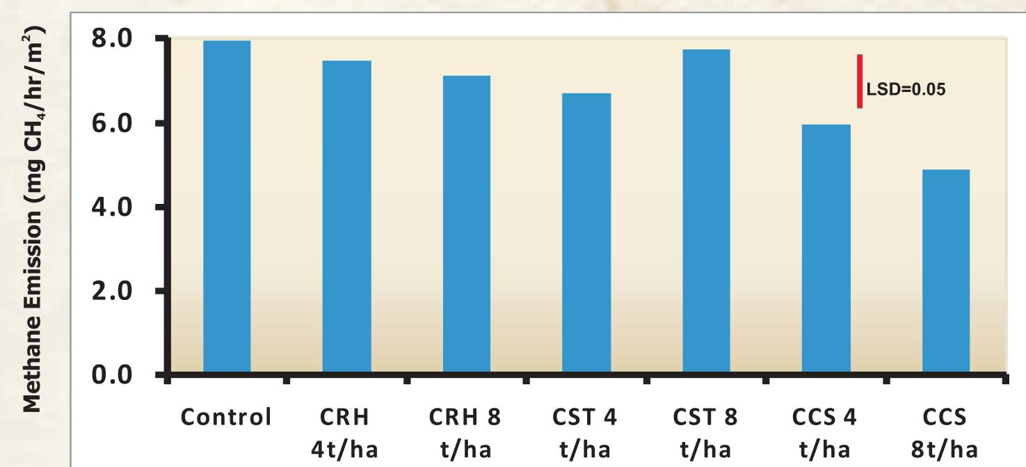
Fig. 1. Application of commercial calcium silicate slag significantly reduced methane emission by 17-22%. This could be attributed by the release of active iron oxide, a source of electron acceptor, eventually resulting in decreased  $CH_4$  emission.
