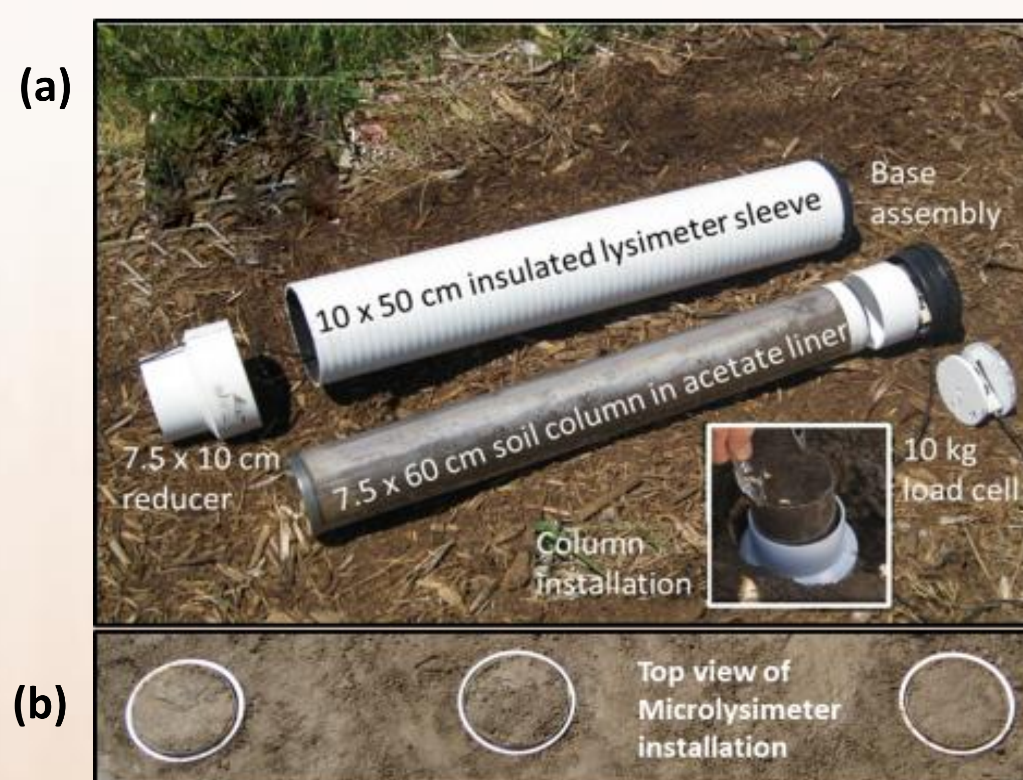
Fig 2: (a) The automated microlysimeter is a 60 mm long soil column housed in an acetate liner and placed on a 10 kg load cell. (b) Field site where microlysimeters were installed.
