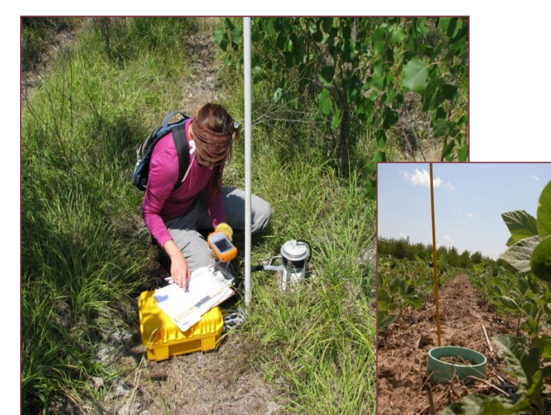
Figure 2. Monthly soil CO 2 , temperature, and moisture measurements taken using an LI-8100 flux system.
