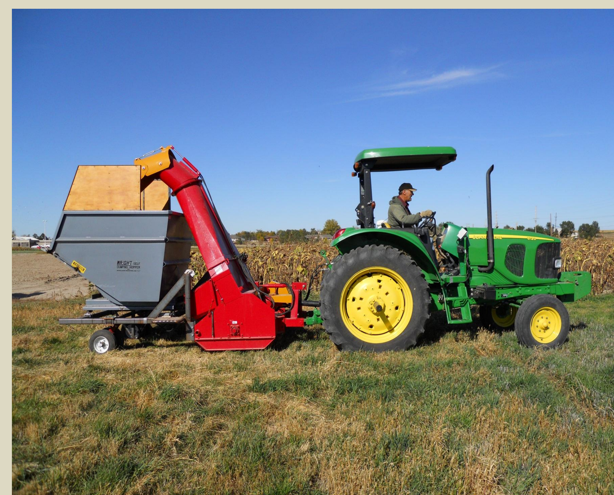
Flail-type plot harvester equipped with self-dumping container and electronic scale.
