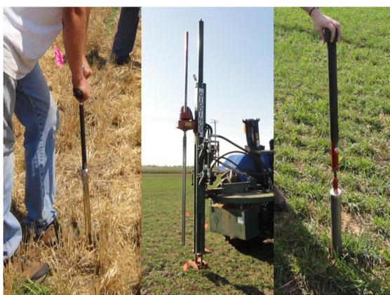
Figure 1: Push, Hydraulic and Slide hammer probe (left to right) with cutting diameter of 2.67, 3.98 and 4.8cm respectively.
