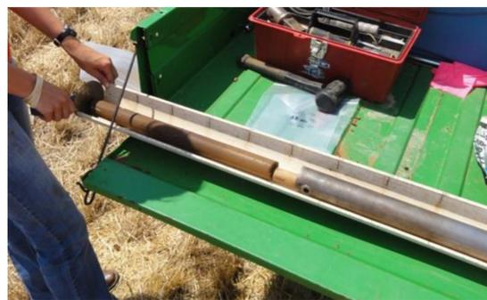
Figure 3: Hydraulic probe core being cut into segments.
