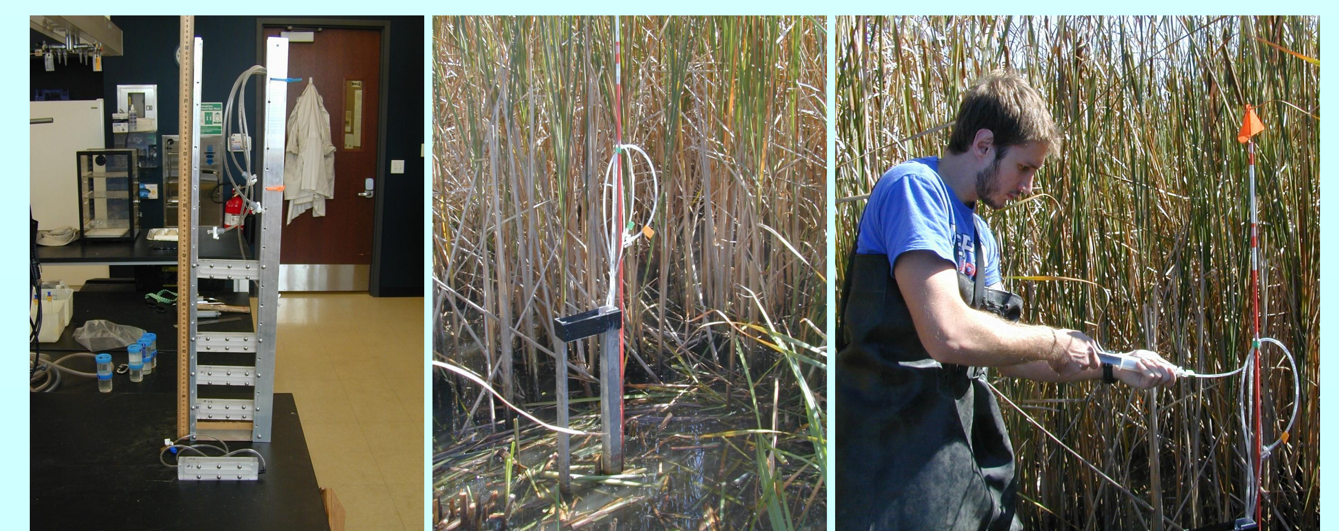
Figure 7: Photos show the diffusion sampler in the lab, deployed at PWS, and during sample collection.
