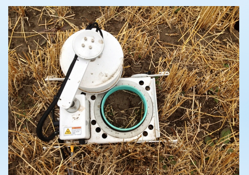
Fig 5. Greenhouse gas (N 2 O, CO 2 & CH 4 ) emissions measured with the Gasmet DX-4015 FTIR-multigas analyzer connected to a Li-Cor 8100-104 long-term flux chamber via a LI-8150-16 multiplexer.
