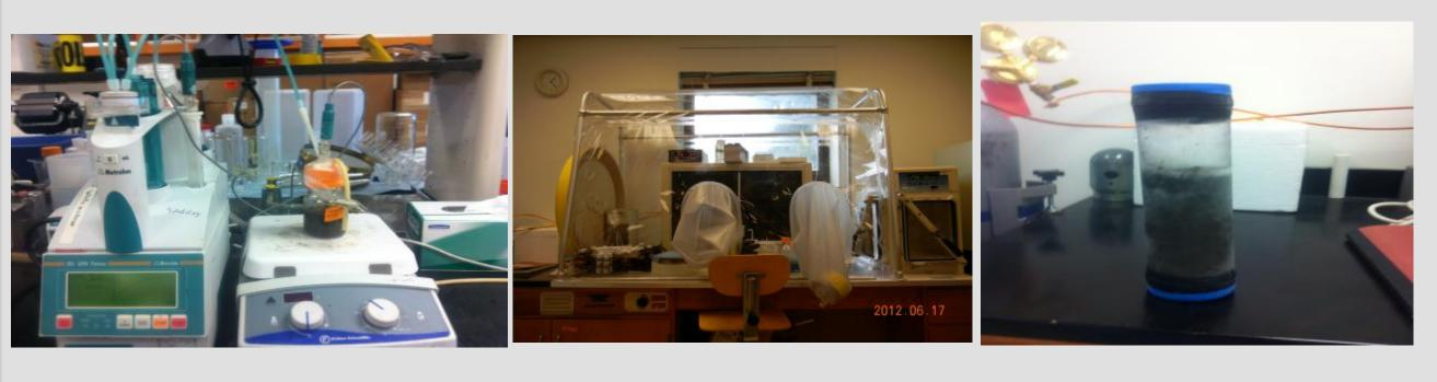
Figure 5: Experimental set up a) pH experiment, b) redox experiment inside glove box, and c) a sediment core from Paul Creek.
