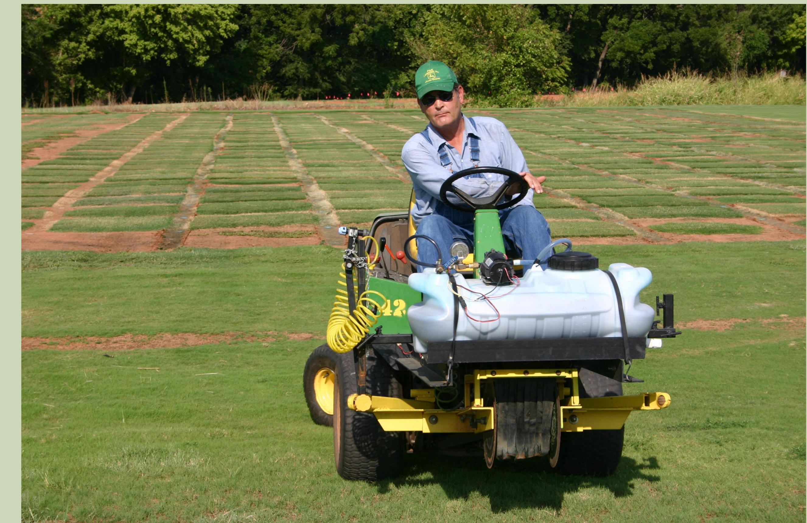
Figure 4: Front view of the combination mechanical slicer-herbicide sprayer device mounted in place of deck on an out-front deck mower. Spray nozzle (not visible) is masked by front flexible spray shroud.
