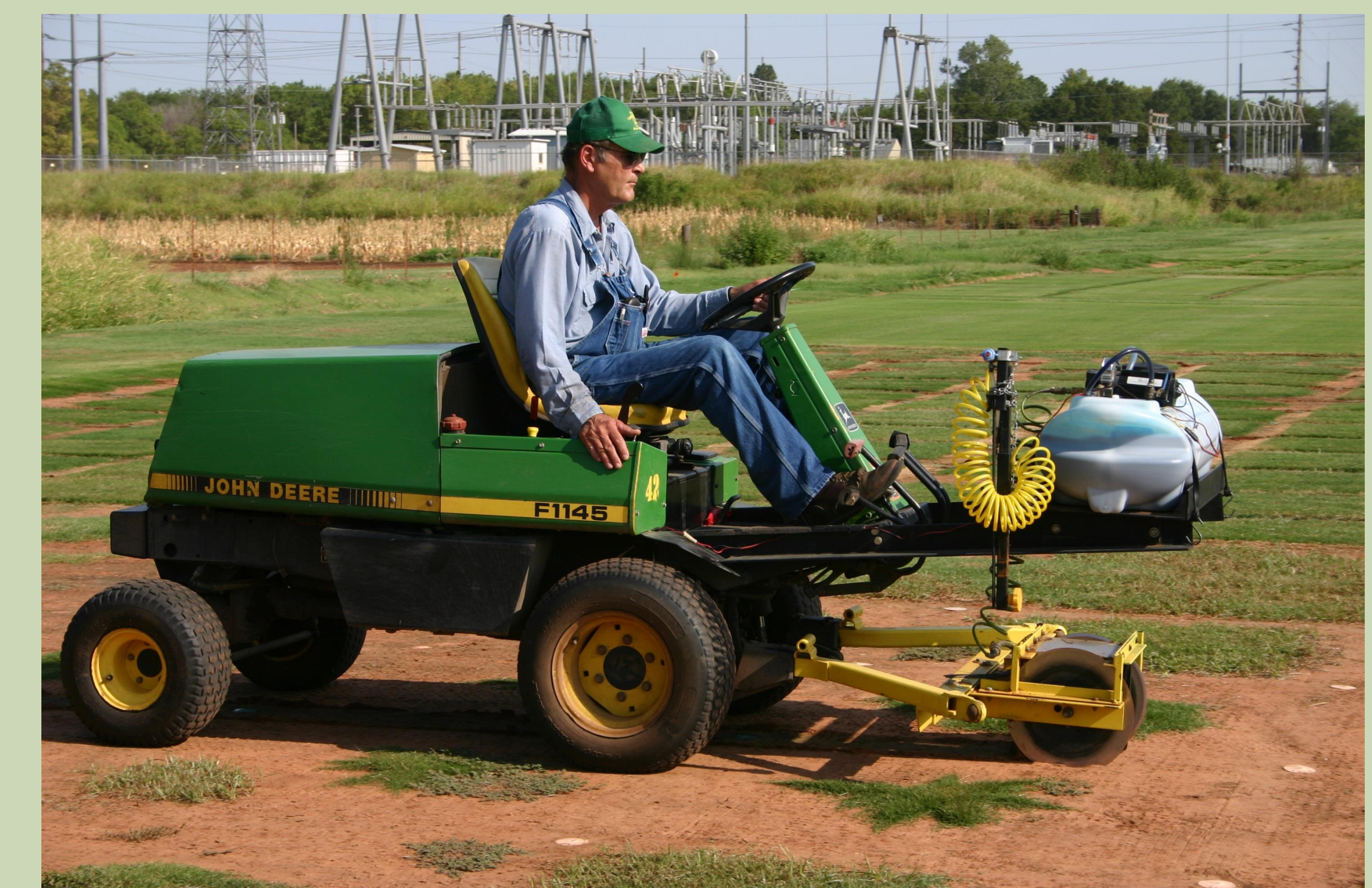
Figure 5: Action view from the side of the combination mechanical slicer-herbicide sprayer device mounted in place of deck on an out-front deck mower.
