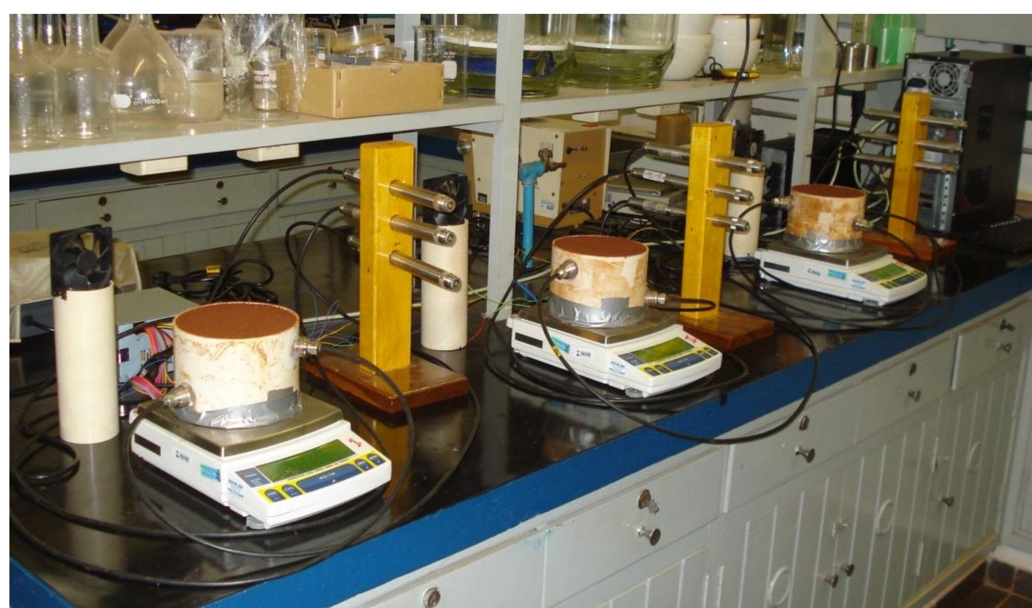
Fig. 2 - View of the evaporation experiment: 3 balances loaded with the rings containing soil and 3 polymer tensiometers each.
