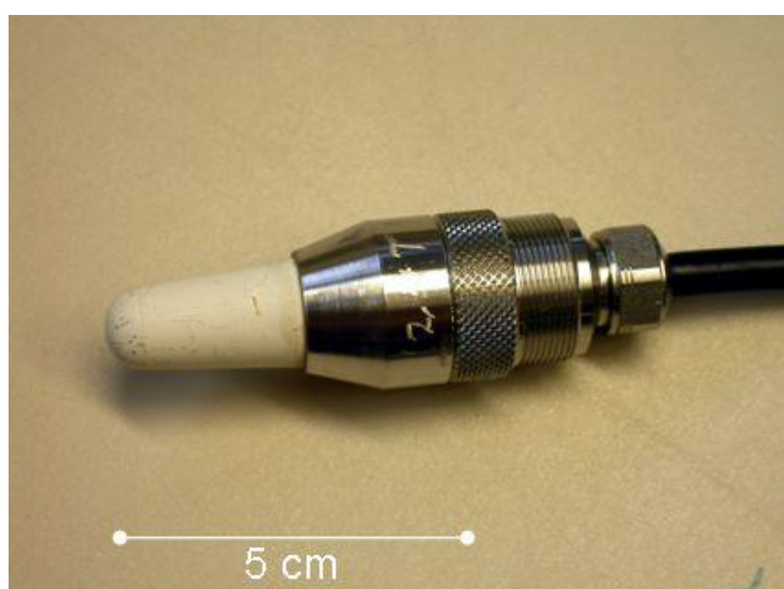
Fig. 1 - Polymer tensiometer cup and polymer chamber. The black cable connects to the datalogger.
