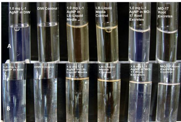
FIGURE 2: A) DIGITAL PHOTOGRAPH OF PARTICLE SUSPENSIONS AT 0 DAYS. Particles are stable in all media, as displayed by the "glow" of the suspension compared to the control media. B) DIGITAL PHOTOGRAPH OF PARTICLE SUSPENSIONS AT 7 DAYS. Particles suspended in DIW and MO-17 Root Excretes remain stable, but those in LB-Liquid Media have aggregated and fallen out of suspension.
