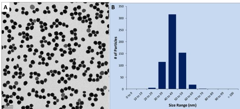
FIGURE 1: A) TEM MICROGRAPH OF AGNPs. Particles are spherical and monodisperse AgNPs. Scale bar is 100 nm. B) PARTICLE SIZE DISTRIBUTION OF AGNPs. Distribution is normal around 40-49 nm, n = 607
