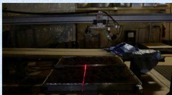
Figure 2. The laser scanner used for experiment.
