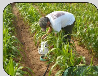
Left: Measuring trace gas emissions from the soil early in the growing season. A LI-COR chamber was integrated with a photoacoustic gas analyzer for gas flux quantification.
