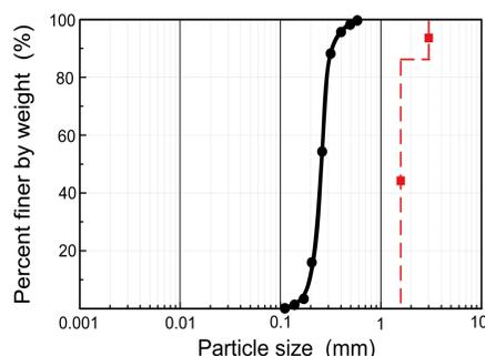
Figure 2. Particle distribution of model soil (red dashed line).
