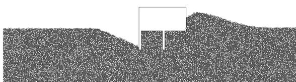
Figure 5. Behavior of model soil under a grouser in DEM ( $\lambda = 0.1$ ,  $h = 4$  cm).
