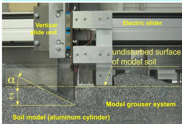
Figure 1. Experimental system using 2D soil model.
