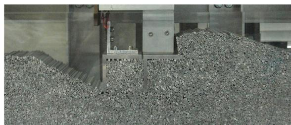
Figure 4. Behavior of model soil under a grouser in experiments ( $\lambda = 0.1$ ,  $h = 4$  cm).
