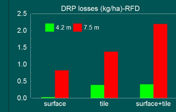
Under RFD system, an increase in tile spacing from 4.6 m to 7.5 m decreased total combined surface and sub-surface flow volume by 12 % but increased both DRP and TP losses. FWM DRP and TP concentrations also increased with wide tile spacing.
