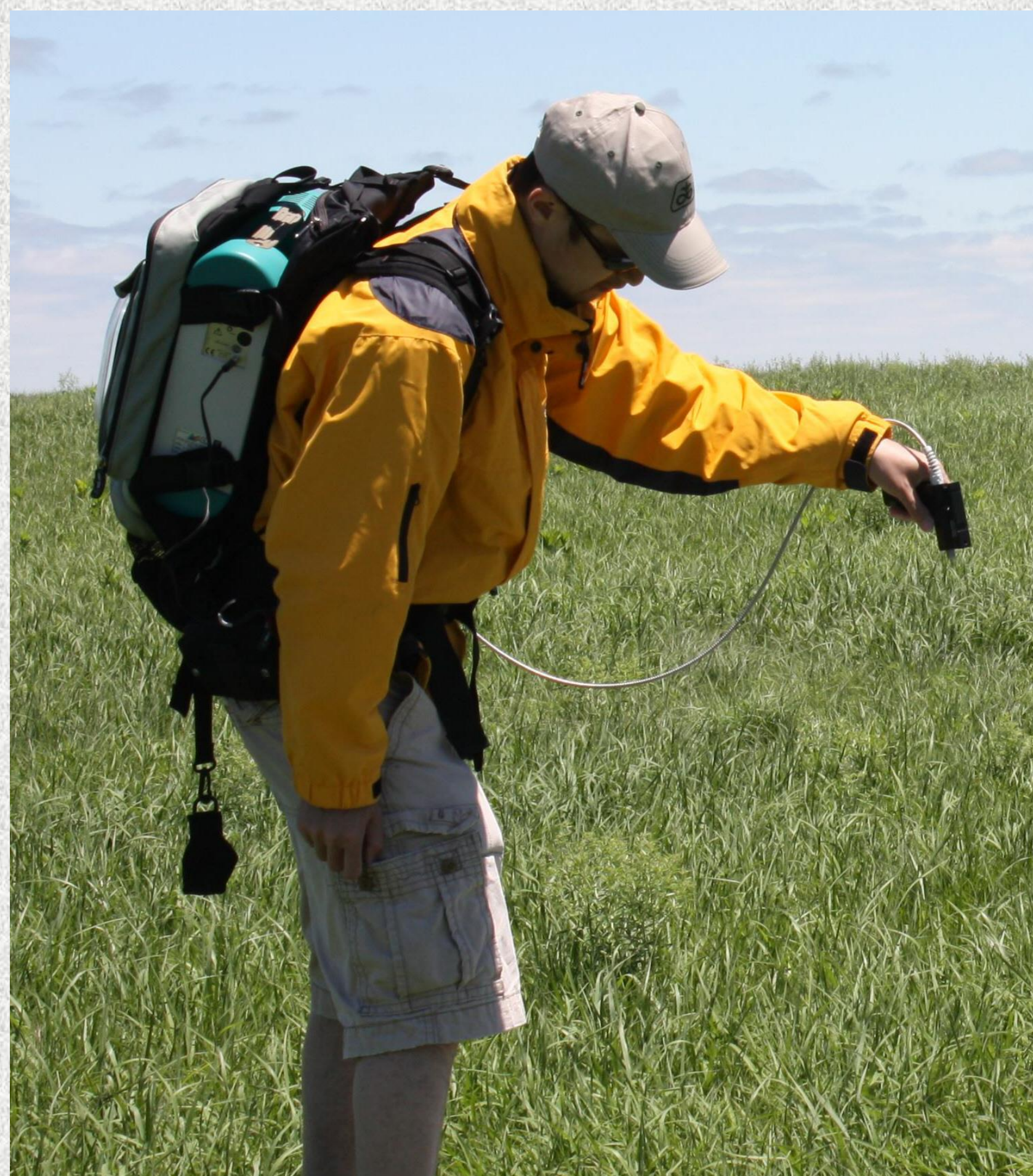
Figure 1. ASD FieldSpec 3 portable spectrometer used to obtain spectral readings from plots.
