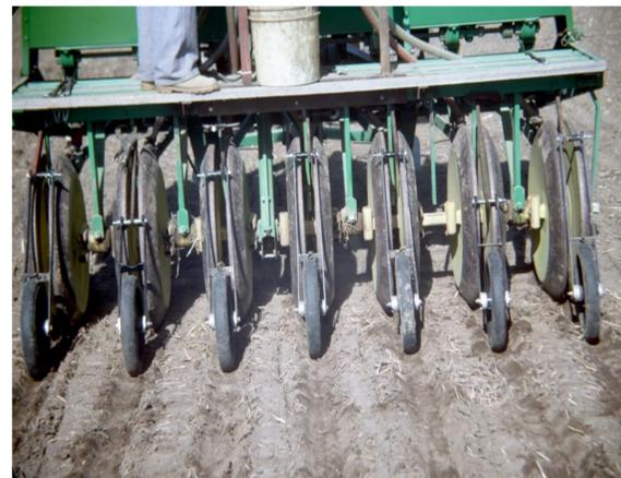
Figure 3. HZ Drill with added packer wheels for planting canola
