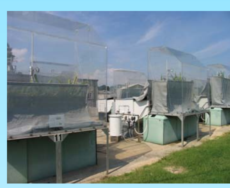
View of corn in growth chambers with curtains to simulate row effects
