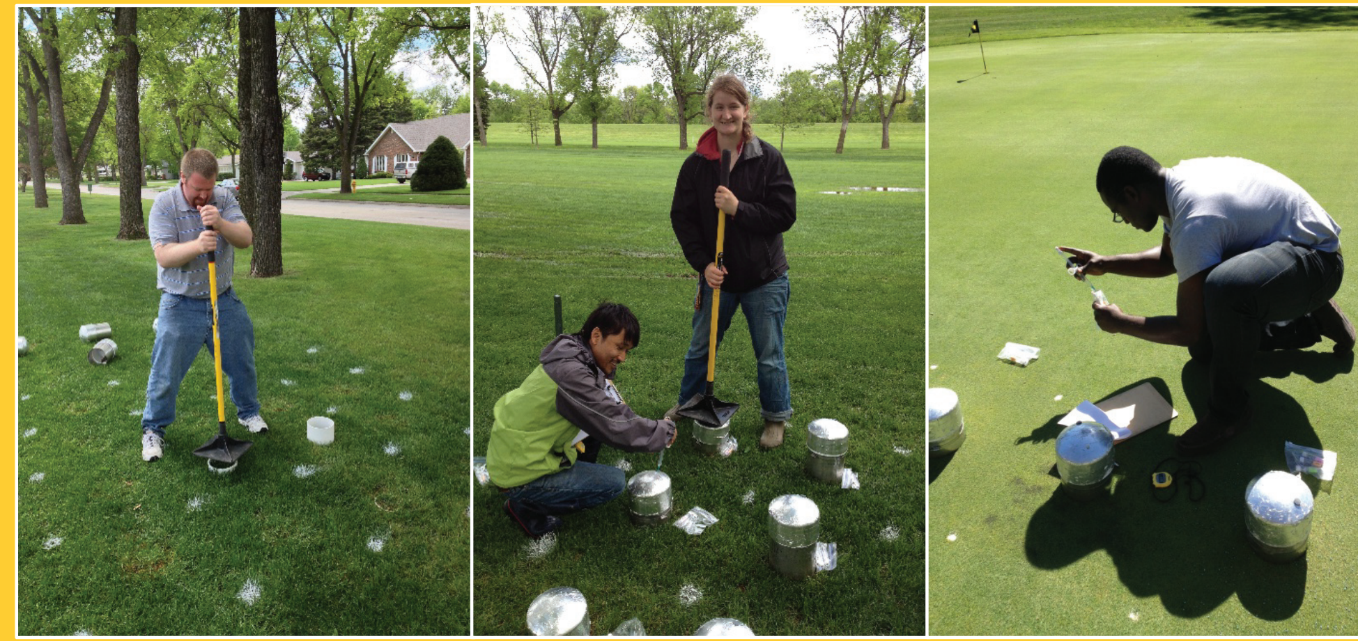
Photo 1: Anchors for each plot were tamped into the soil at the beginning of the study to provide a base for the gas chambers. Photo 2: Prior to sampling for greenhouse gases, the gas chambers were tamped onto the anchors to create a good seal. Photo 3: Gas samples were taken at 0, 20, and 40 minutes post closure of the gas chamber and another.
